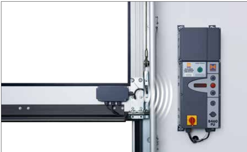
Radio transmission unit To transfer the signals from the door leaf to the control via Bluetooth (no coiled cable), power supply via a powerful battery; connectable components: optosensors LE (low energy), leading photocell VL 1-LE / VL 2-LE, 8k2 strip, cable slack switch, wicket door contact, night latch contact
